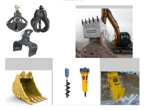
Use the correct attachment for the task, do not use the attachment for any other purpose than it is intended for.
